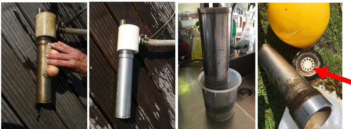
*Cleaning mesh filter with brush and/or soaking filter in acetic acid*
