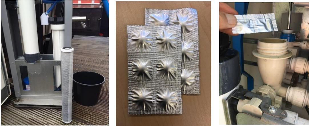
*Remove AC filter and add Chlorine Dioxide tablets in the dispenser*
