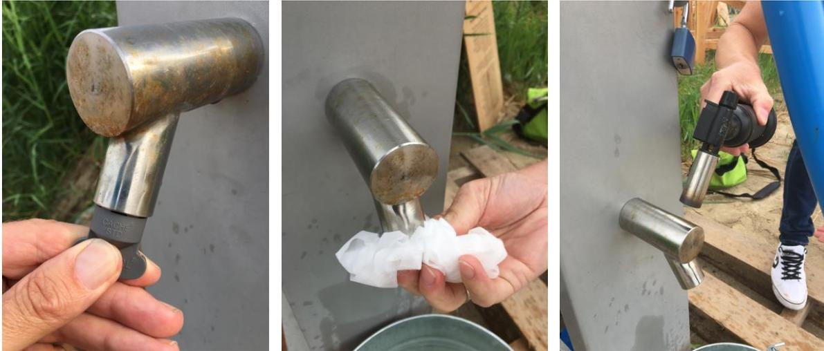
*Removing flow gauze, disinfect tap and flaming the tap*
