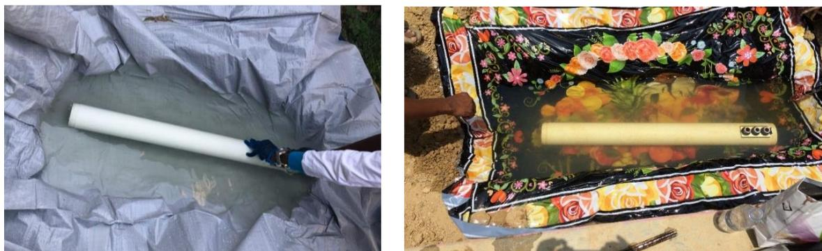
*How to clean the membrane in the field? for example making a bath with chemical solution, by digging a hole in sand and cover this with a waterproof blanket.*
