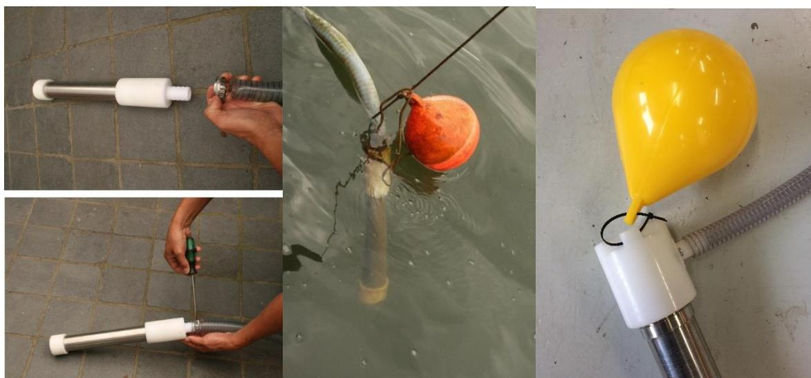
*Mounting the Mesh Filter to the hose; connect the floater to the Mesh Filter with for instance a tie wrap in order to keep Mesh Filter just below the water surface. If there is no floater available you can also use an empty can or bottle.*
