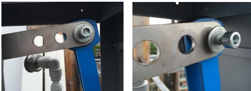
*Fork installed at third hole of lever.*
