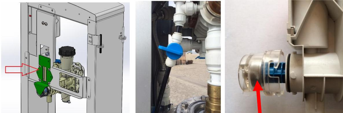
Remove the metal valve cover, open the blue tap to release pressure (and close again) and remove the transparent piston cover
