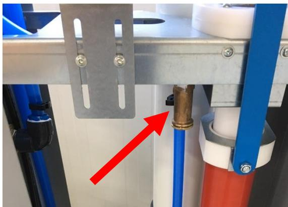
*Pressure relief valve: releases water if the pressure at the UF membrane has exceeded 0,7 bar and/or when pumping during backwash*
